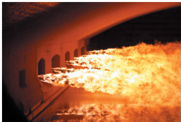
Float batch is melted using the heat generated through the combustion of fossil fuels
